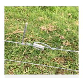
This is an example showing poor use of a crimp. It should be crimped properly, then the ends wrapped around the main wire on each side of the crimp at least twice, then snapped off leaving no sharp ends. This also shows poor knot tying - the correct knot would be a figure 8 or crimp to join the wires.
